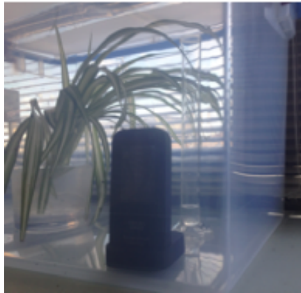
Figure 5. This shows the setup of the spider plant, formaldehyde meter, and formaldehyde source (originally 10 mL of formaldehyde in a graduated cylinder) in the sealed plastic container (inset). Graphical representation (bottom).
